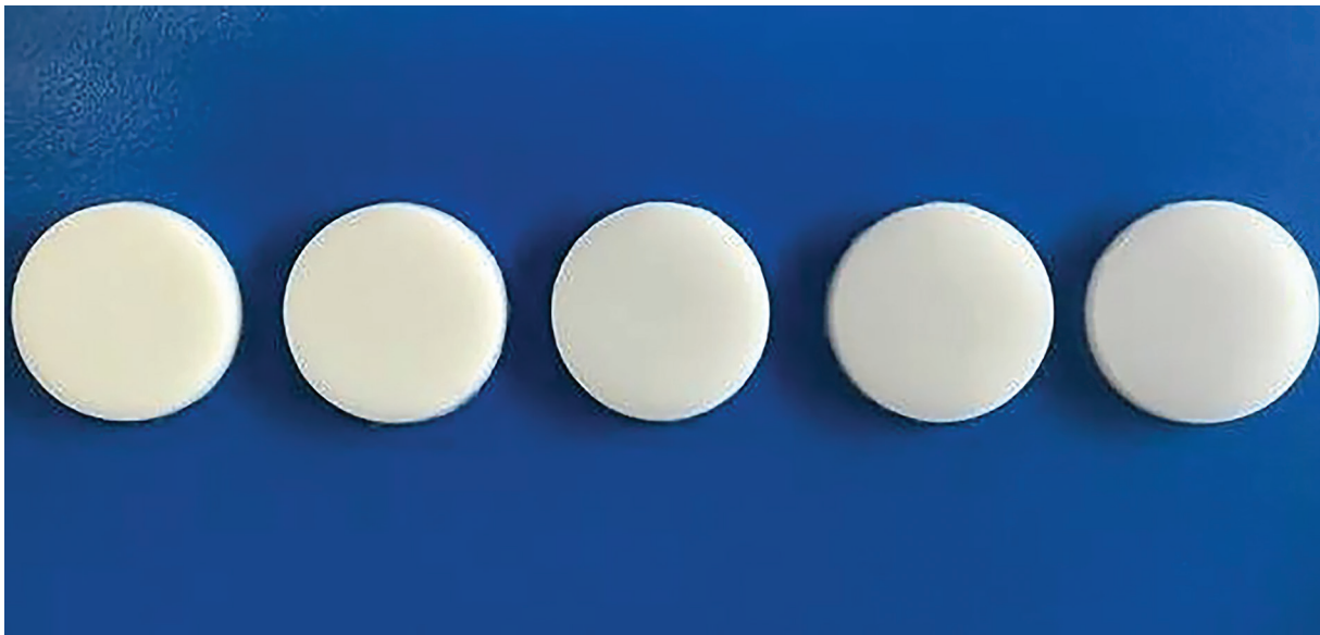
Fig. 1 Specimens of silicone with 0.2% functional intrinsic white, 0.5, 1, 1.5, and 2% nano zinc oxide by weight (from left to right).
