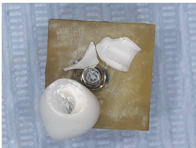
Fig. 3 Multiple fractures of the zirconia abutment above the platform.
