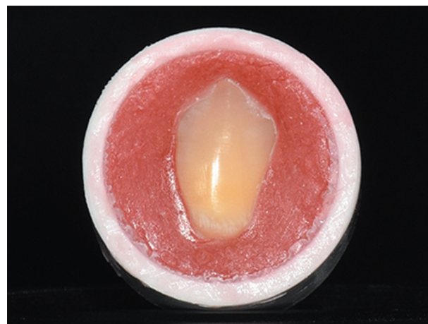
Fig. 1 Human maxillary first premolar crown embedded in a plastic pipe and fixed by self-curing acrylic resin with its buccal surface 1.0 to 1.5 mm above the pipe rim.
