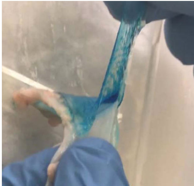
Fig. 1 Tough adhesive demonstrating strong adherence to porcine dura during peel-testing.
