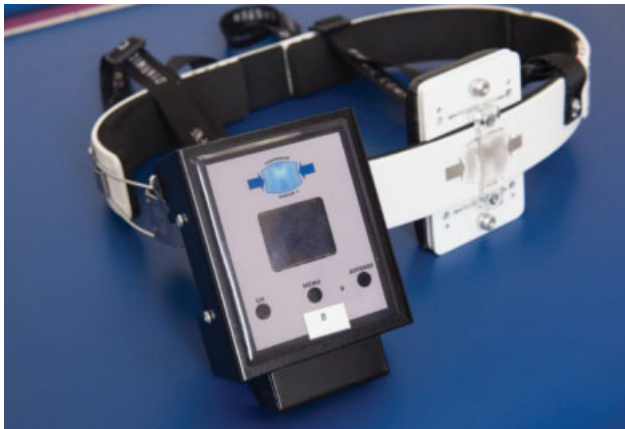
Fig. 1 Dynamic compression system (DCS) and pressure measuring device.
