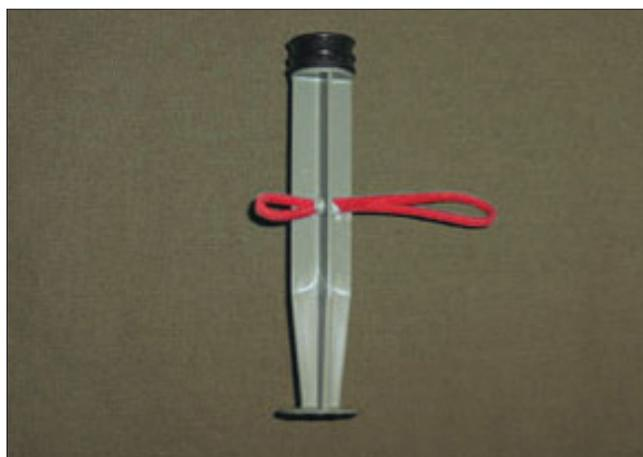
**Figure 2:** The rubber band is passed through a hole in the 5 cc piston to form small loop and a big loop
