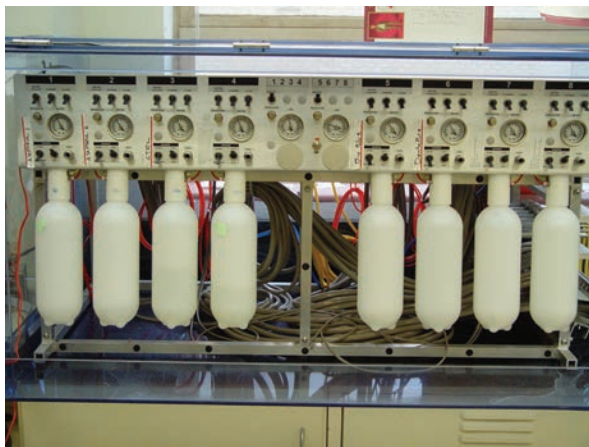
Figure 1A. Front view of the automated dental unit simulator showing 8 dental unit water systems with pressure gauges and manual control switches.
