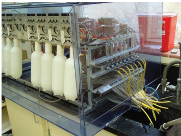
Figure 1B. Side view showing effluent end of waterlines (4 handpiece & 1 Air/Water Syringe per each of the 8 dental unit water systems) and pneumatic controls.
