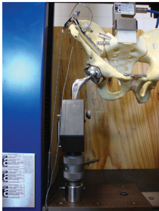
Fig. 4 The right iliac bone was connected to the lower head of the machine by means of two steel cables (diameter 1.6 mm) that simulated the gluteus medium muscle for pelvic stabilization. The cables were attached to the ilium with the aid of a plate. One of the cables was attached at the level of the iliac crest and the other to the anterior gluteal line, near the tubercle of the iliac crest.
