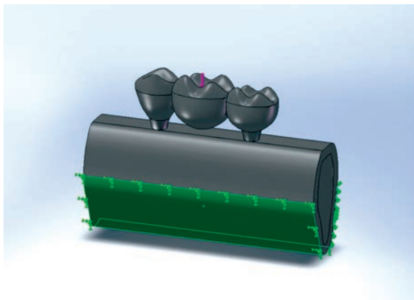
Figure 3b. Load application and boundary condition of veneering porcelain. The pink arrow represents the load application, and the green area is assumed to be fixed as a boundary condition.
