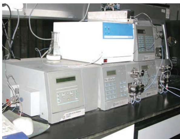
Figure 2. The High Performance Liquid Chromatography (HPLC) apparatus employed in the present investigation.
