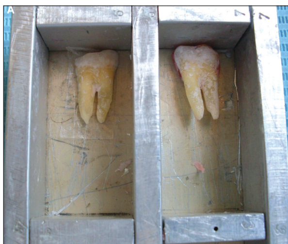
Figure 1A. The control specimen lied on its dentin side on double face adhesive tape (left) while the experimental specimen lied on double layer of pink wax to create artificial acrylic walls. Both specimens surrounded by a metallic rectangular mould on which the self-cured acrylic resin was poured.
