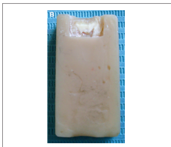
Figure 1B. The experimental specimen after hardening of the acrylic resin material shows the specimen surrounded by three artificial acrylic walls.
