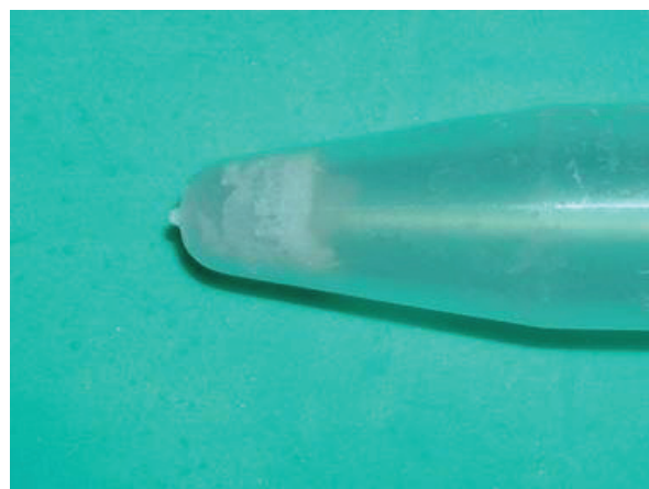
Figure 2. Appearance of salt deposit and dry debris in a centrifuge tube.
