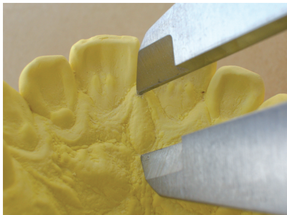
Figure 1. Measurement of the distance between most anterior and posterior borders of the incisive papilla on stone casts.
