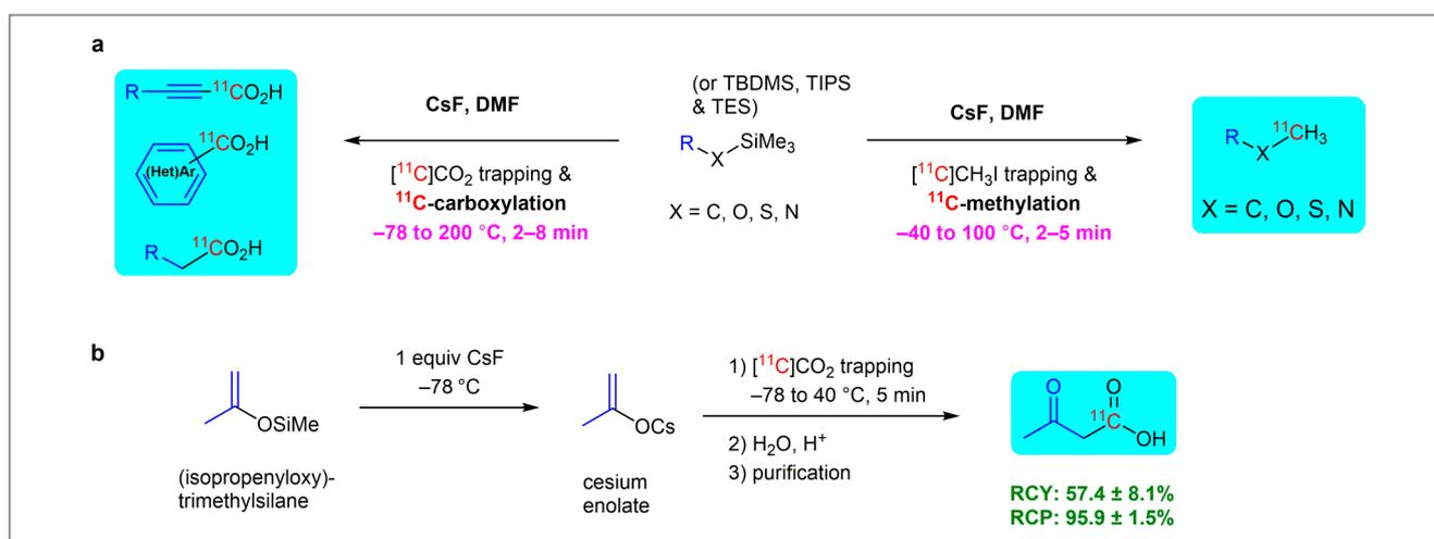
**Scheme 1** Fluoride-mediated desilylation for (a)  $^{11}\text{C}$ -carboxylation and  $^{11}\text{C}$ -methylation of organic molecules and (b) FMDS  $^{11}\text{C}$ -carboxylation for synthesizing  $[^{11}\text{C}]\text{acetoacetic acid}$ .
