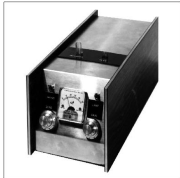
Fig. 2 The first Born aggregometer. The instrument equipped with a stirring device and galvanometer was presented during a workshop at the Royal College of Surgeons in 1961. Of note, changes in the optical density had to be read and subsequently plotted manually (→Fig. 3). (taken from Born 14 and reproduced with permission of the Born family).
