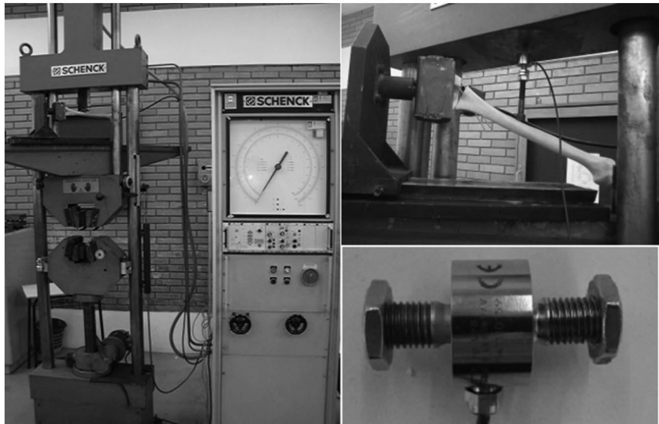
Fig. 3 Universal tensile testing machine model UPM 200 and an HBM U9B load cell (20 KN = 1 mV/V)
