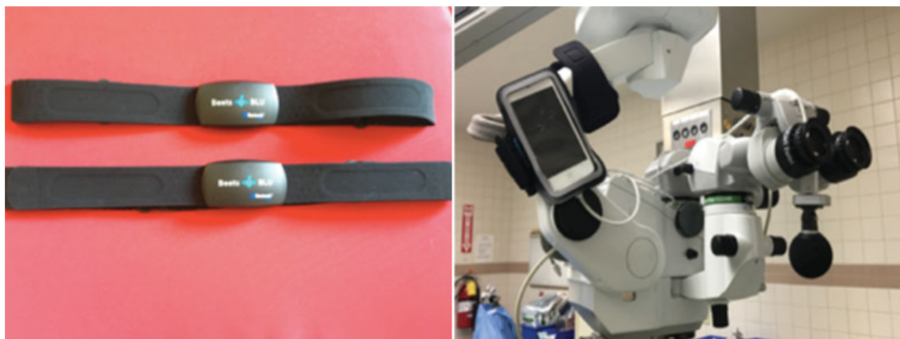
Fig. 1 Beets BLU chest-strapped Bluetooth devices (left) and the setup showing placement of microphone and iPod device on the microscope (right).
