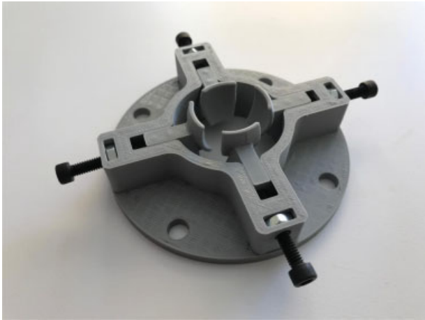
Fig. 4 Table-top globe holder for ex vivo imaging.
