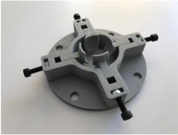
Fig. 4 Table-top globe holder for ex vivo imaging.
