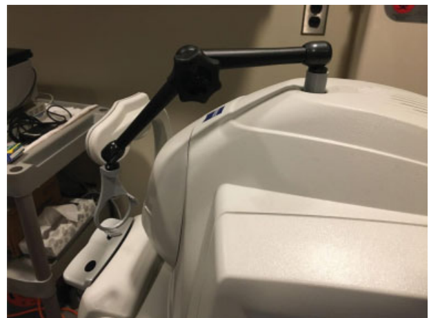
Fig. 3 OCT-mounted lens holder for an accommodation study.
