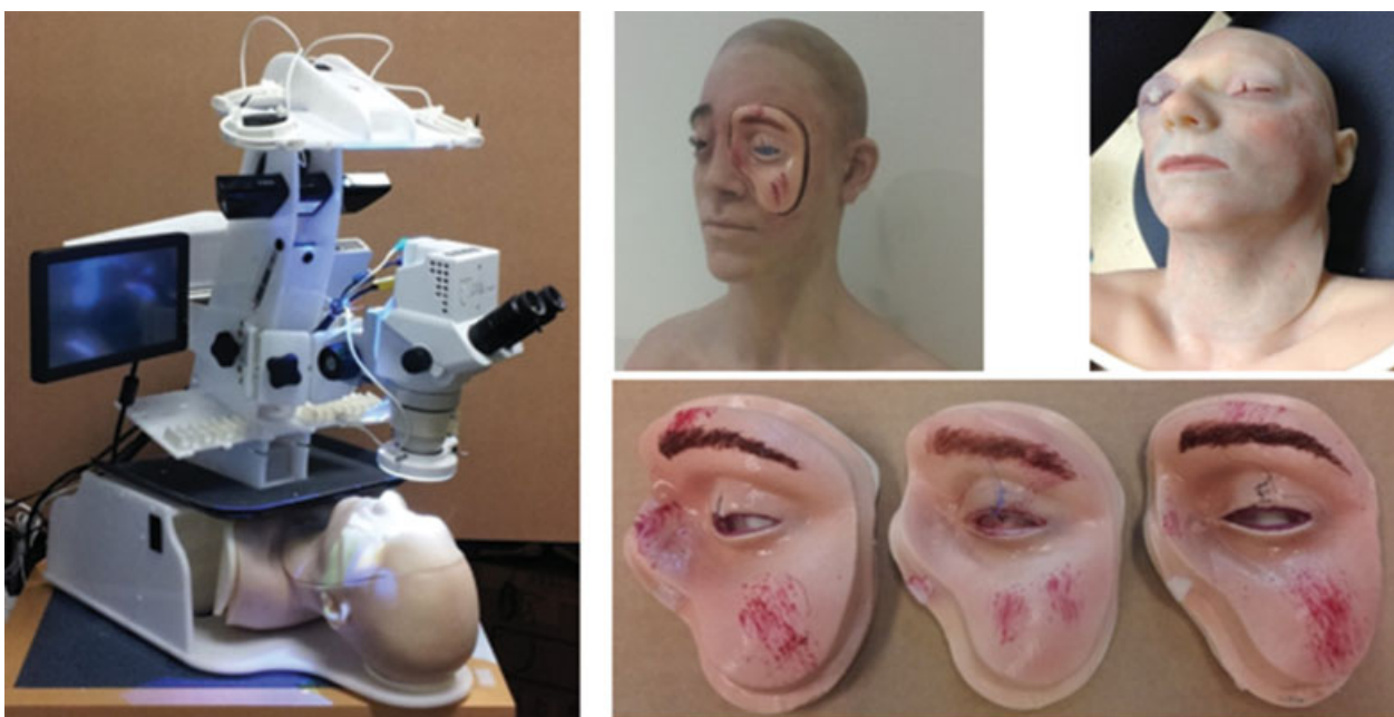
Fig. 2 Ocular and Craniofacial Trauma Treatment Training System with optional microscope attachment.
