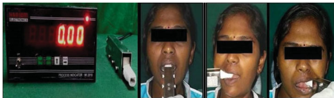
Fig. 1 Showing digital bite force recorder and bite force measurements at the central incisor, right first molar, and left first molar region by using bite force recorder.
