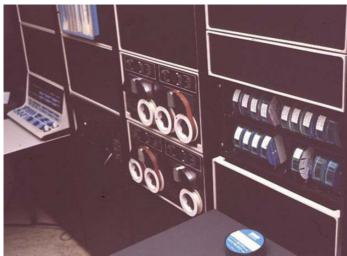
Fig. 1 The PDP-15 computer that we used in the early 1970s for our research in electrocardiology. It had four DEC-tape readers for the storage of data and programs, and operated with 'words' of 18 bits.
