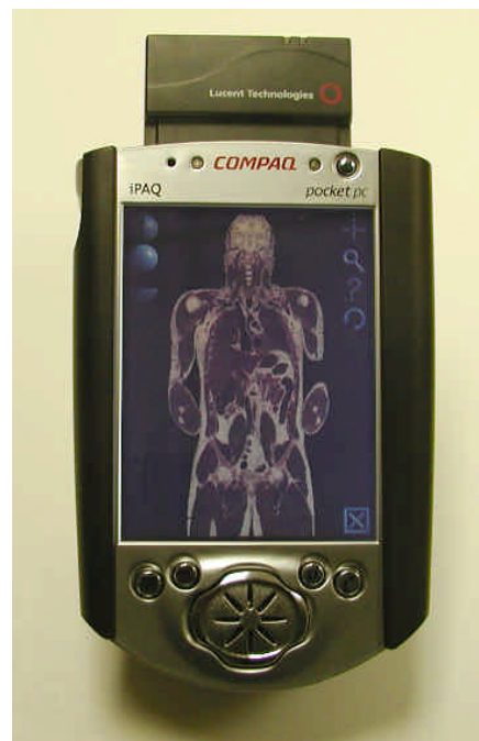
Fig. 3. The handheld device displays a slice through the Visible Human Male data. The data reside on a server at the University of Wisconsin, La Crosse, and can be accessed interactively by remote devices over the Internet. This image is computed by placing a cutting plane through a stack of horizontal cross-sectional images.
