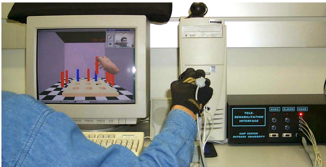
Fig. 2. The VR-based orthopedic rehabilitation using a haptic glove during a peg-board exercise. © IEEE 2000. Reprinted by permission.
