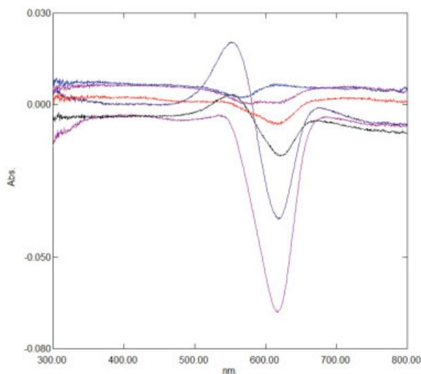
**Fig. 3** Difference spectrum of 50  $\mu$ M MV in 20 mM citrate buffer pH 4.0 with control added to the reference cuvette and *Glycerol* 50 M added to the sample cuvette. Spectra correspond to  $t = 0$ ,  $t = 10$  minutes,  $t = 100$  minutes,  $t = 260$  minutes,  $t = 4$  days and  $t = 11$  days after mixing (see text for details). MV, methylene violet (Berntsen).
