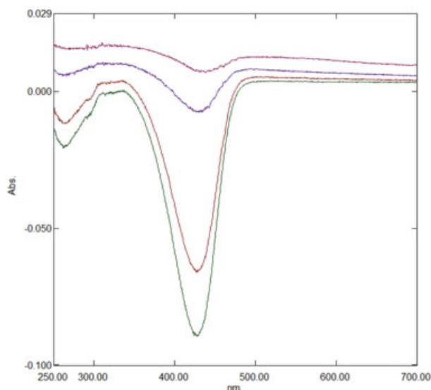
**Fig. 4** Difference spectrum of 50  $\mu\text{M}$  C343 in 20 mM phosphate buffer pH 7.0 with control added to the reference cuvette and *Glycerol* 50 M added to the sample cuvette. Spectra correspond to  $t = 17$  minutes,  $t = 150$  minutes,  $t = 12$  hours and  $t = 7$  days after mixing (see text for details). C343, coumarin C343.
