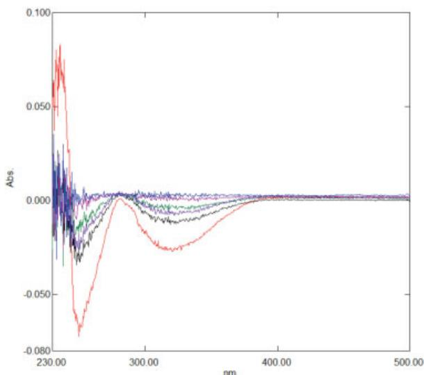
**Fig. 7** Difference spectrum of 200  $\mu$ M ANA in 20 mM citrate buffer pH 3.5 with control added to the reference cuvette and *Glycerol* 50 M added to the sample cuvette. Spectra correspond to  $t = 0$ ,  $t = 10$  minutes,  $t = 40$  minutes,  $t = 100$  minutes,  $t = 200$  minutes and  $t = 4$  days after mixing (see text for details). ANA, 6-amino-2-naphthoic acid.
