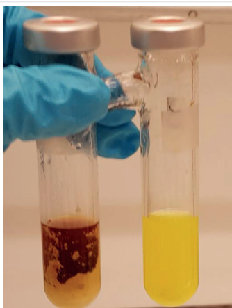
Figure 2 Two-Chamber vial after radical carbonylation reaction. Left-hand chamber ( C_{CO} ) contains DBU/Mo(CO) 6 , right-hand chamber ( C_{rxn} ) contains reactants. 34
