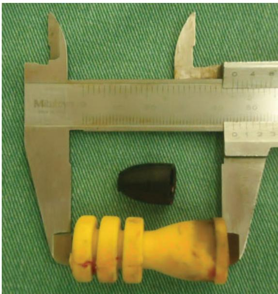
**Fig. 5** Image showing projectile size, its outer yellow rubber coating, and the core.
