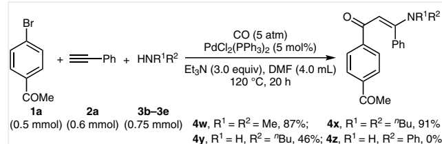
Scheme 4 Palladium-catalyzed carbonylative addition reactions of various amines
