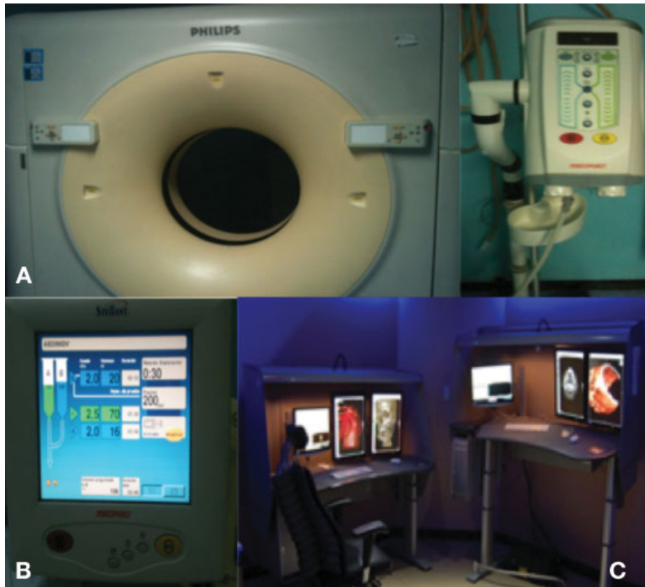
Fig. 2 CT suite. (A) 64-slice multislice computed tomography with power injector. (B) Contrast medium administration device. (C) Picture archiving and communications system (PACS).
