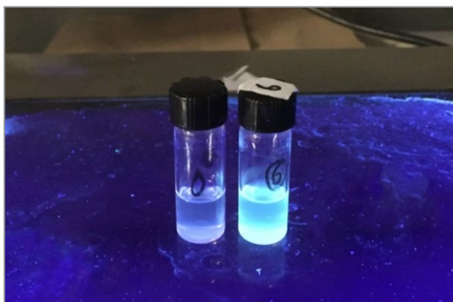
Figure 2 Fluorescence responses of FI-DIBO to sodium azide in a tea sample; FI-DIBO 100 \mu M, NaN 3 (1.12 mg/cup) in a mixture of tea solution and dioxane (1:1) at pH 7.4
