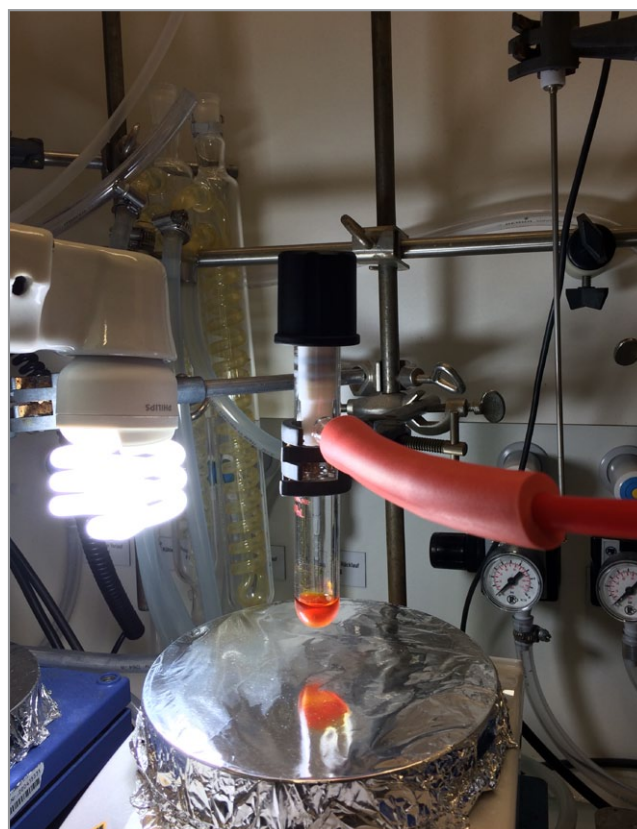
Figure Exemplary photochemistry setup using a compact fluorescent lamp
