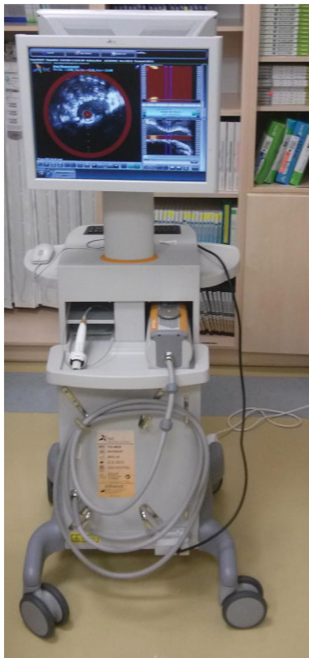
Fig. 1 The near infrared spectroscopy imaging device consisted of the following three main parts: a dual-modality 3.2 F imaging catheter that incorporates both near-infrared spectroscopy and intravascular ultrasound; a device for the mechanical pullback and rotation of the catheter through a vessel; and finally, a console with which one can observe the results of both imaging modalities in real time in the catheterization laboratory.
