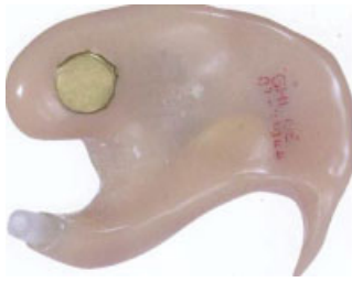
Figure A2 Photograph of second-generation sound generator shell.
