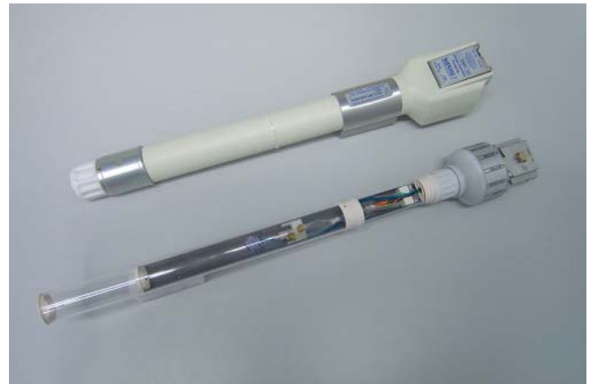
Fig. 4 Two technical support units (TSU) are shown. The upper TSU will be attached to the MPI positioning system. The lower one is used for MRI measurements. It has a mounted mouse carrier unit which can be locked by a screw. Both TSUs feature connectors and interfaces for narcotics, air for the heating system, and vital sign derivation.
