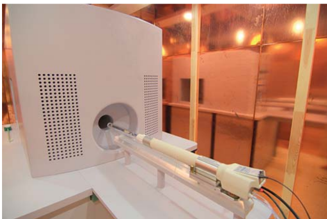
Fig. 1 Preclinical Magnetic Particle Imaging scanner is installed in a shielded cabinet. The copper coating shielding eliminates disturbances induced by external radio frequency signals. The scanner has a circular bore (diameter ~12 cm). With the positioning system, the animal carrier unit, which is fixed to the technical support (TSU), can be pushed into the bore. All tubes and cables for narcotics, air for the heating system, and vital sign derivation are attached to the TSU and are piped to the carrier unit.
