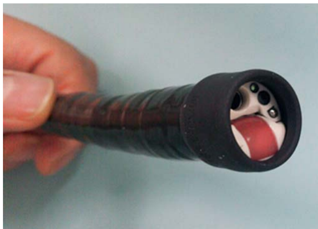
Fig. 1 To solve the difficulty of tumor scanning and scope fixation during endoscopic ultrasound-guided fine-needle aspiration of a small gastrointestinal subepithelial lesion (SEL), a cap device is attached to the tip of a forward-viewing and curved linear-array echoendoscope scope tip; this device fixes the SEL.
