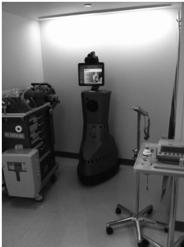
Fig. 1 Example of RP-7 robot in community emergency department used for acute stroke teleconsultation staffed by a large university center.
