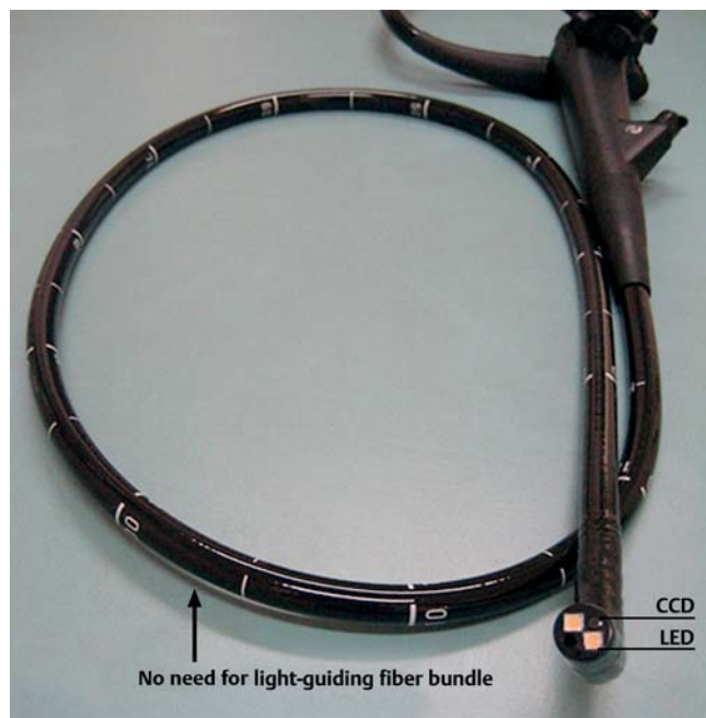
Fig. 1 The prototype high-definition colonoscope illuminated by light-emitting diodes (LEDs). Two packages of white LEDs are attached to the distal end of the colonoscope. The colonoscope has no need of a large light source apparatus and light-guiding fiber bundle. High-definition images and image-enhanced endoscopy using flexible spectral imaging color enhancement are available. CCD, charge-coupled device
