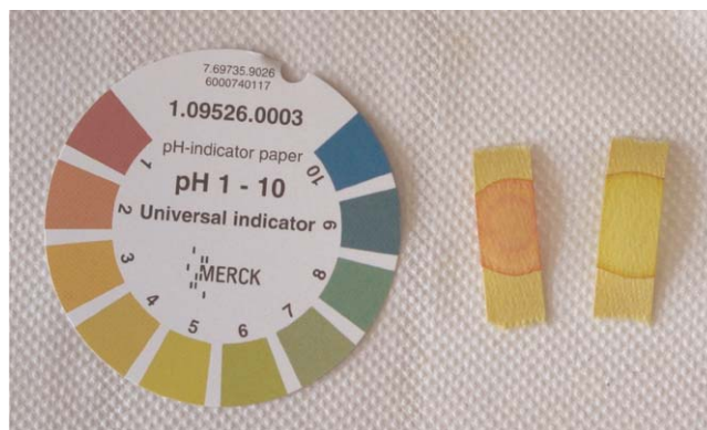
Figure 3 Testing the different batches of TRIP with pH paper. Left: type B , right: type A .
