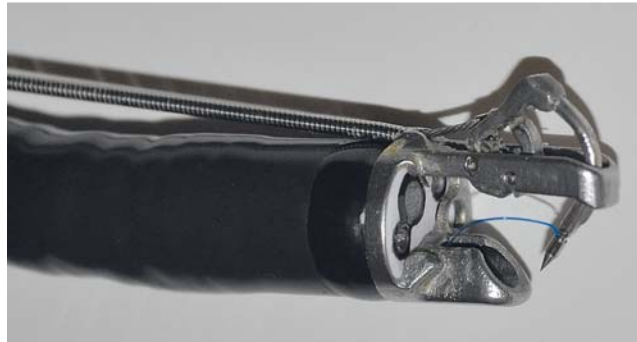
Fig. 1 The distal part of the endoscopic suturing device, mounted onto the tip of a dual-channel endoscope.
