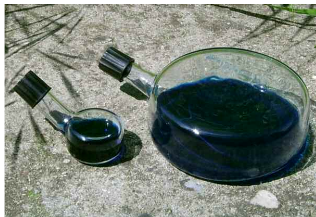
Figure 1 Photocatalyzed reaction: the blue color demonstrates the presence of reduced catalyst P\text{-H}
