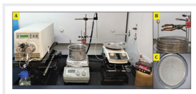
► Fig. 3 (A) Continuous flow setup for the synthesis of CPC; (B) Hastelloy coil reactor (1/8" OD, 10 mL internal volume capacity) used for conducting the experiments; (C) in-house CPC synthesized through continuous flow.
