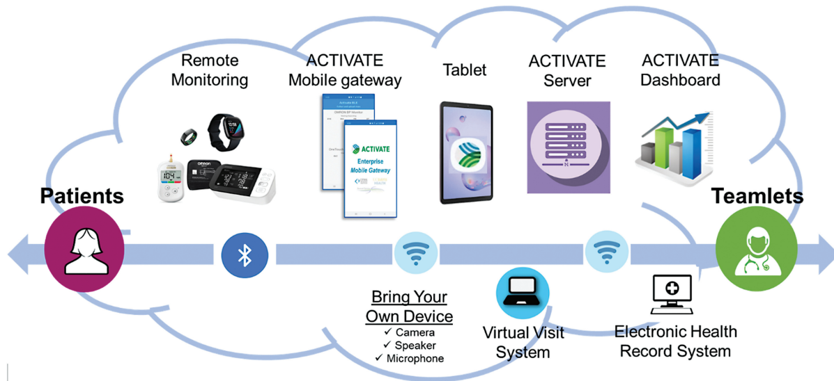
Fig. 1 ACTIVATE digital health platform. The figure depicts the digital health solution for rural patients with diabetes and hypertension. The RPM devices connect via Bluetooth to a mobile gateway app on a tablet (or bring your own device) connected via the Internet to the server. RPM data flow to the dashboard and a weekly data summary is deposited as a document in the EHR. Virtual visits are scheduled in the EHR and conducted by the patient on the tablet. EHR, electronic health record; RPM, remote patient monitoring.
