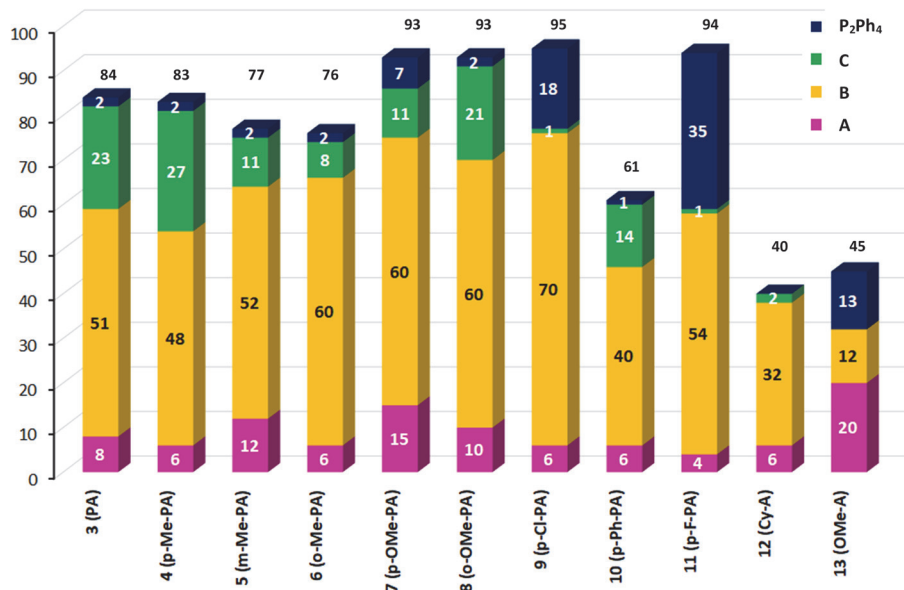
Figure 2 Substrate scope for the hydrophosphination of allenes with HPPH 2 using pre-catalyst 1 . Conditions: 0.6 mmol allene, 0.5 mmol HPPH 2 , 0.025 mmol 1 , 0.6 mL C 6 D 6 . Conversions determined by inverse-gated 31 P NMR spectroscopy with PPh 3 as an internal standard and reported relative to HPPH 2 . Total conversion shown above each column. See the Supporting Information for further details.
