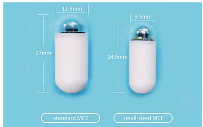
► Fig. 1 Comparison of a standard magnetically controlled capsule endoscopy (MCE) device and the small-sized MCE device (both Ankon Technologies Co., Ltd., Wuhan, China).
