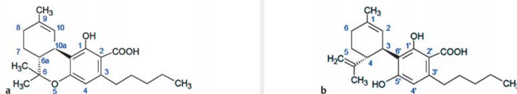
► Fig. 1 Δ 9 -Tetrahydrocannabinol acid THCA (a) and Cannabidiol acid CBDA (b) are the target cannabinoids in medicinal cannabis. By decarboxylation at C-2 they are inverted to the pharmacological active constituents in medicinal cannabis.
