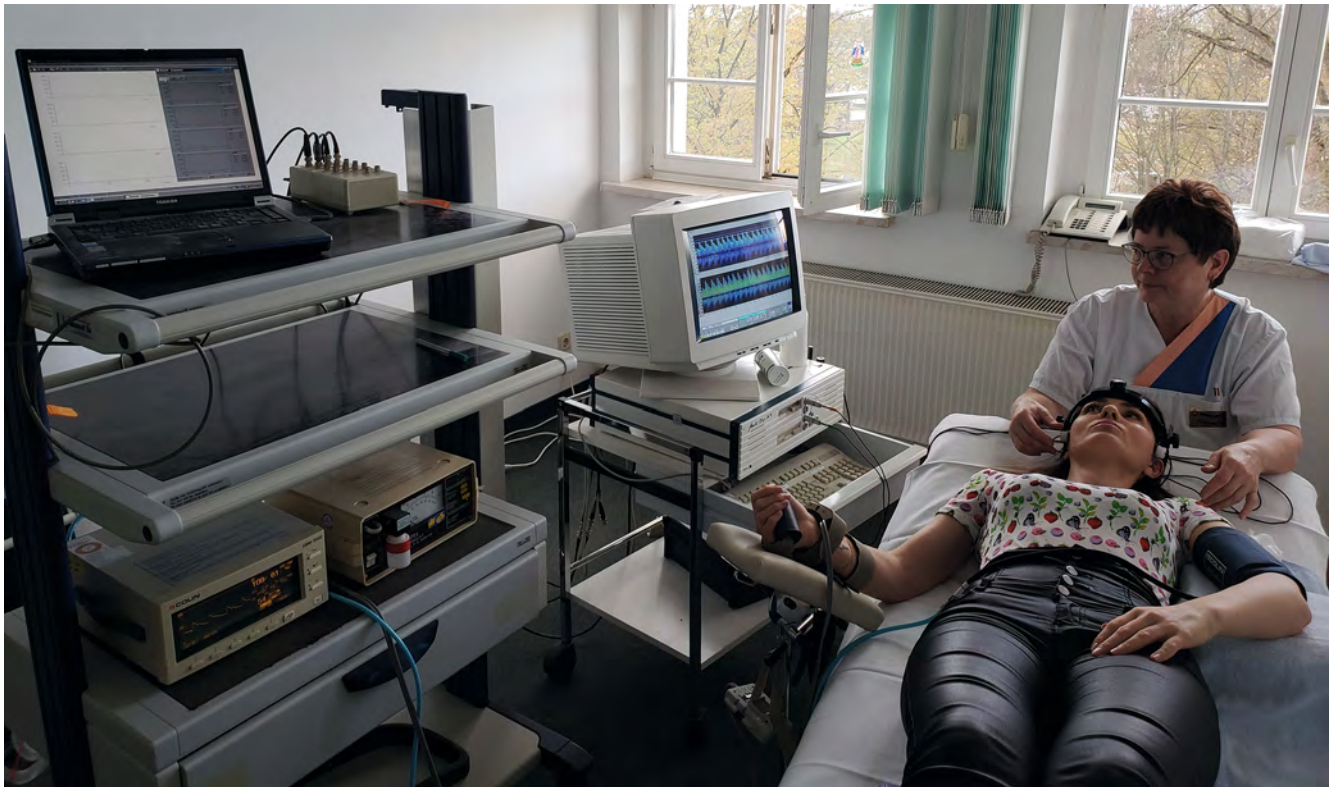
► Fig. 2 Study workup. The study workup is presented by two employees of our hospital. The ABP pressure sensor is mounted at the right radial artery of the patient, and the pressure cuff for ABP mean value calibration is located on left upper arm. Both of them are connected to the Colin ABP device (bottom left). The left upper arm is elevated to keep the cuff at head level. Two TCD monitoring probes fixed by a headset are located for bilateral insonation of the MCA. The analog output signals of both the ABP and the Doppler device (in the middle) are connected to a laptop (top left) and converted into digital signals, which were stored and displayed on the monitor using our in-house software. At the time the picture was taken, mask wearing was not required in our hospital.
