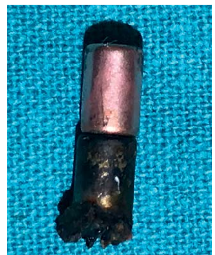
► Fig. 3 Photograph of the removed magnets showing corrosion on one side.
