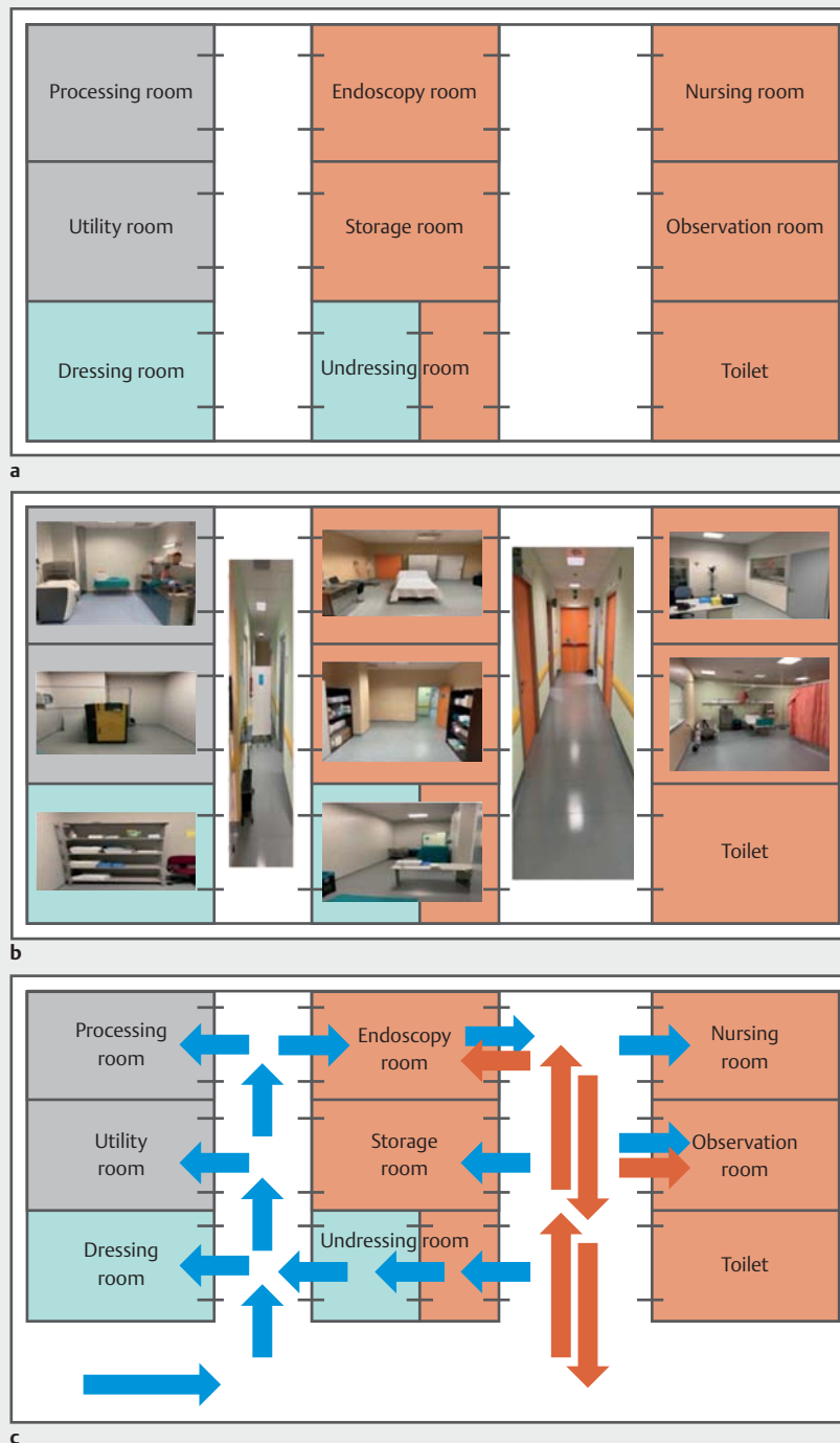
► Fig. 1 Unit plan for the endoscopy service created at Niguarda Hospital, Milan, Italy, for the treatment of patients with COVID-19. a The rooms are colored to show the three different areas: clean area in green, unclean area in red, and the “gray” area (not completely clean, inaccessible to patients). b Photographs of the rooms in the plan. c Pathways of movement for patients and healthcare workers. The blue arrows show the unidirectional path for healthcare workers; the orange arrows show the path for patients.
