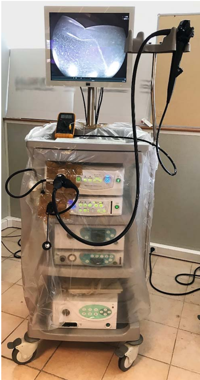
► Fig. 3 Endoscopic system with a plastic film around the light source and the processor box.
