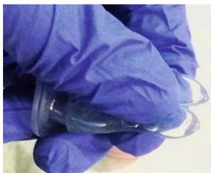
► Fig. 2 A silicon nipple with a slit functions as a valve.
