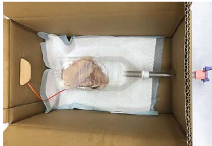
► Fig. 1 Setting the skinned chicken meat with an electrode in a 2-L polyethylene terephthalate bottle.
